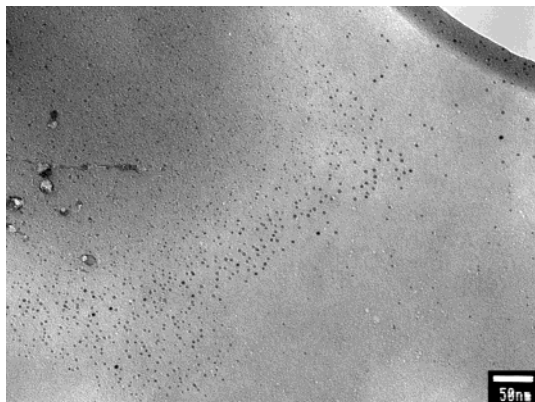
Figure 3. TEM micrograph of \alpha -Mo 2 C nanoparticles annealed briefly at 600 °C.
